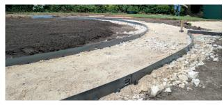
All of the edgings except our weathered steel (Cor-Ten effect) have a 20-micron Galvanised Zinc coating. Our (RAL) coloured edgings have a further 110-micron UV resistant polyester powder coating preventing colour fade, forming a durable scratch resistant barrier guaranteeing a 20yr plus product life.
